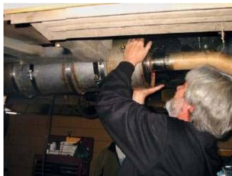
Installing a catalyzed diesel particulate filter (DPF) is nearly as simple as replacing the muffler. DPFs are extremely effective and remove over 90 percent of diesel exhaust particles. These filters can typically be installed on 1994 and newer vehicles that have electronic engine systems.
