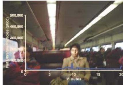
In-coach levels of ultrafine diesel particles in this test were 10-100 times higher in coaches being pulled by a locomotive (left) than in coaches being pushed (right).
