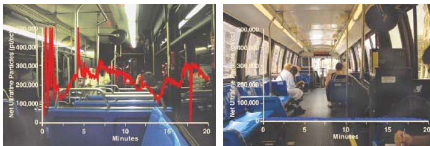
Left: Pollution from a conventional bus infiltrates the cabin exposing passengers to elevated levels. Right: Diesel ultrafine particle pollution from the bus is undetectable in the cabin of a bus with a DPF.
