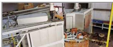
GameTime began its molding operation with a single rotational molder, a Ferry Industries 430 Model, in 1982 with only three colors available and six operators. Today, those numbers have increased to four Ferry machines, three shifts, 38 operators and 16 standard colors. The 220, 280, 430 and 500 Ferry models go through 4 million pounds of LLDPE a year, with the 280 and 430 acting as the work horses of the four.
